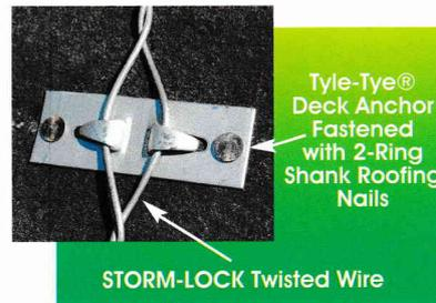
Individual roof tiles are tied into the loops of the Tyle-Tye® Twisted Wire by means of a Tie Wire or Tie Rod of similar metal. Besides being anchored at eave and ridge the Tyle-Tye® Twisted Wire system is anchored at 5 foot intervals as required to avoid overstressing any one anchor point.
